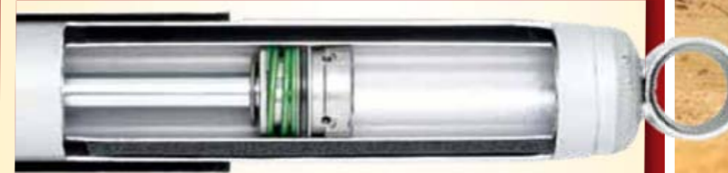
The foam lining in the outer tube helps combat shock fade by keeping the gas and oil separate
