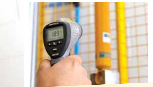
The maximum temperature was measured at the start and finish of each dyno run. The temps were slightly higher compared to the real-world testing where the shock is exposed to airflow when the vehicle is moving
